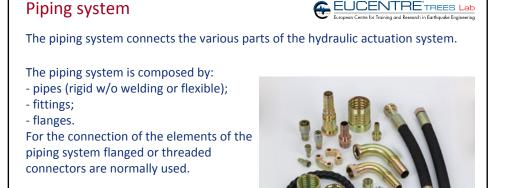
The design of the components of the piping system must be performed depending on the working and peak
